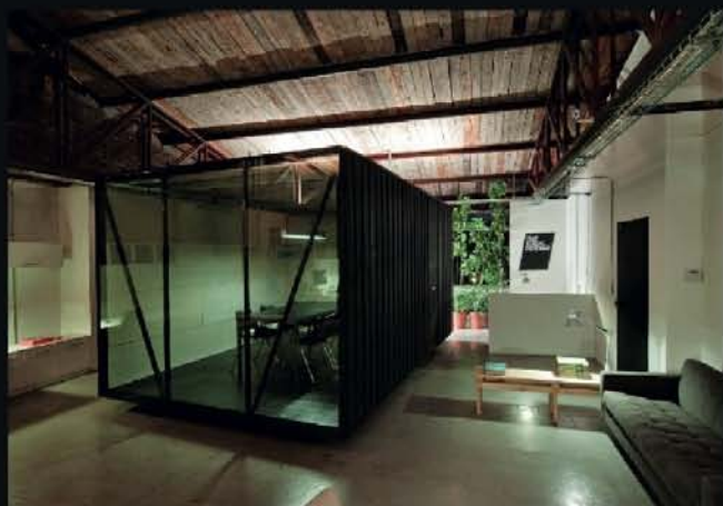
Left Pre-painted corrugated sheets were used to clad the exterior of the conference room
